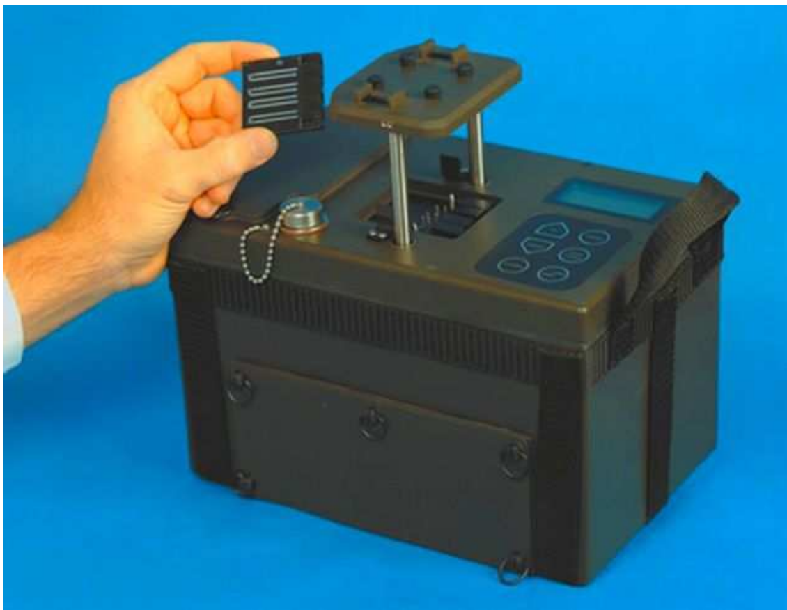
Figure 2: Fiber-optic biosensor from Naval Research Laboratory (Washington, DC) for environmental monitoring of hazardous chemical or biological materials and has undergone extensive field testing.
